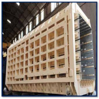
WIL delivered critical assemblies of Trisonic Wind Tunnel at VSSC (ISRO)
